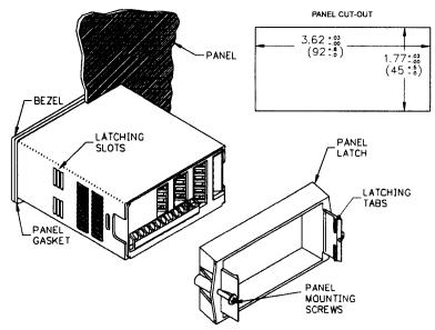
Figure A.2. Installation of the display in a panel.
