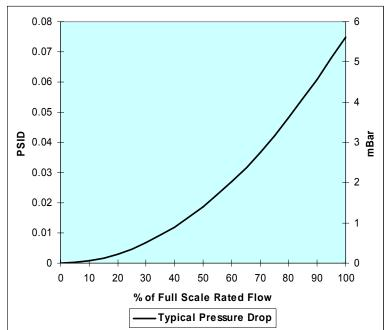
Pressure Drop vs. Percentage of the Full Scale Rated Flow for the Model 50 Series
