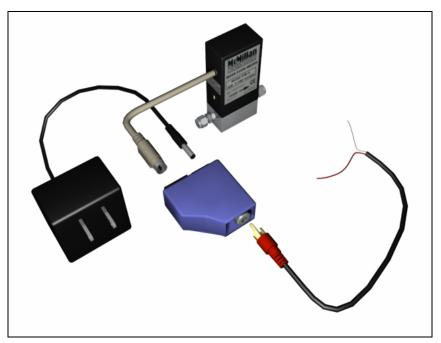
A 0-5VDC analog output proportional to the flow rate may be made available by connecting the cable assembly to the connection hub. This output may then be connected to a display, data acquisition system or voltmeter with an impedance of greater than 2.5 k $\Omega$  (kilo ohms).
