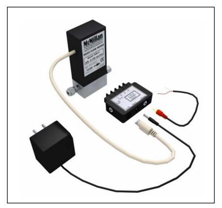
A 4-20mA analog output proportional to the flow rate may be made available by connecting the cable assembly to the connection hub. This output may then be connected to a display, data acquisition system or current meter.
