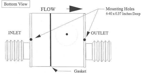
Approx. 2.13 Inches between mounting hole centers Compression forces on the gasket must be maintained between mounting brackets.
