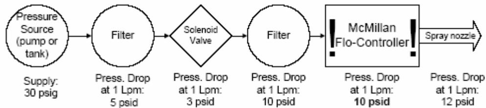
This system starts with 30 psig of supply pressure but other components (minus the flow controller) total 30 psid. This leaves no pressure for the flow controller. Either the supply pressure would have to be increased, and/or a source of pressure drop (such as the post-pump filter) would need to be eliminated:
