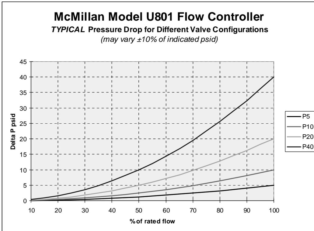
Note: the P5 and P10 control from 20-100% of the maximum rated flow. All other configurations control from 10-100% of the maximum rated flow.
