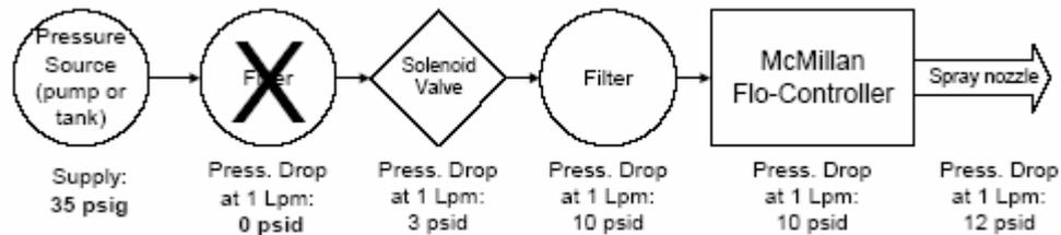
The system now has 10psi available to operate the flow controller. If the supply pressure was 40psi then there would be 15psi available to operate the controller.
