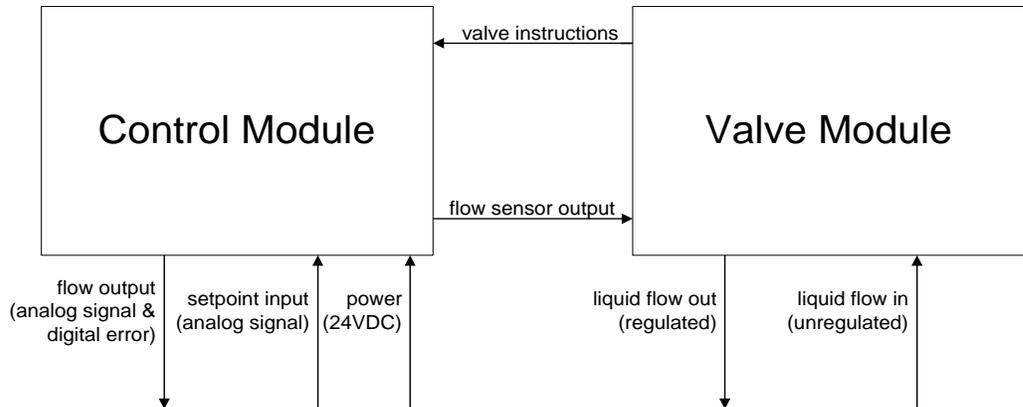
The above diagram shows the logic used by the Flo-Controller to measure and control flow rate as desired.
