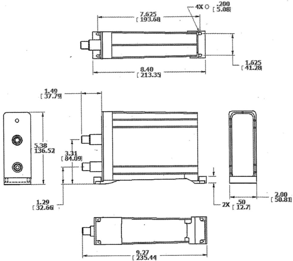
Dimensions shown are in inches(mm). All dimensions shown are for Model U802 FLO-CONTROLLER with 3/8" male flare fittings (F6) and are similar for other models. Specific model dimensional drawings may be requested from the factory.
