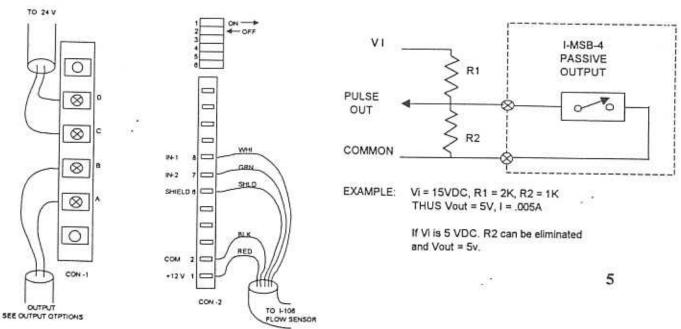
Pulse output height is approximately Vi x (R2/(R1+R2)). Keep Vi < 36 vdc. Be sure that Vi / R1 does not exceed 20 ma.
