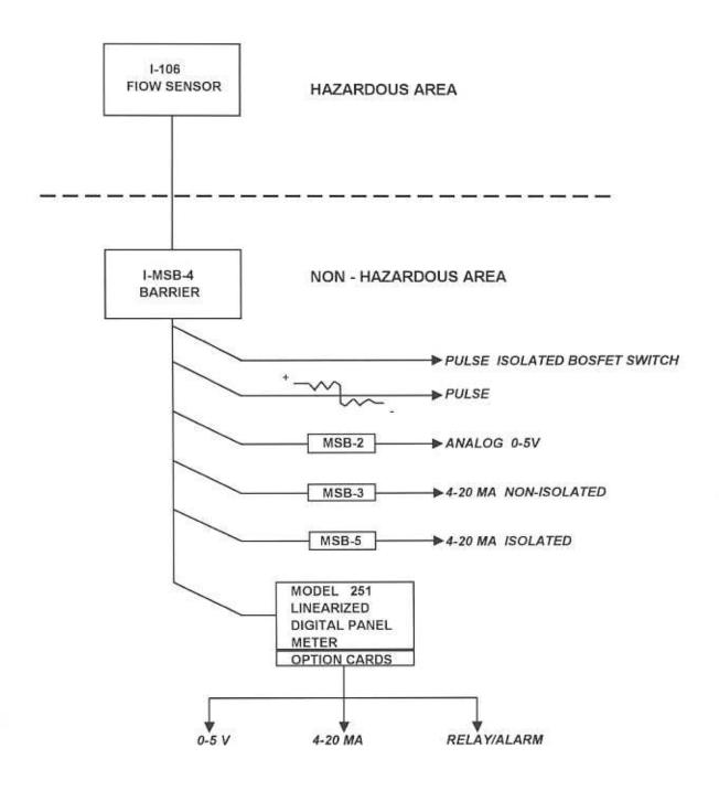
ANY OF THE ABOVE OUTPUT OPTIONS, WHEN TAKEN FROM THE OUTPUT OF THE I-MSB-4, OPERATES AS PART OF THE USER DATA ACQUISITION SYSTEM AND THUS DOES NOT AFFECT THE INTRINSIC SAFETY OF THE FLOW SENSOR SYSTEM.
