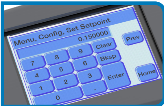
ON-SITE VALVE SET-POINT ADJUSTMENTS
